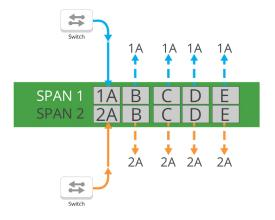
In this scenario you are able to ensure 2 SPAN ports provide 1-4 copies of unidirectional traffic each, without packet injection back onto the network.
