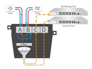
In this scenario you are able to TAP one link and provide unidirectional 'filtered' tap copies of traffic, without packet injection back onto the network.
