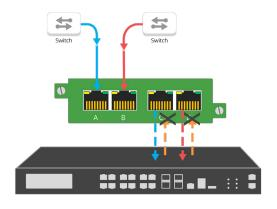
In this scenario you are able to ensure 2 SPAN ports provide 1 copy of unidirectional traffic each, without packet injection back onto the network.
