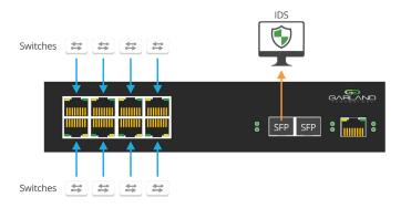
In this scenario you are able to ensure 8 SPAN ports provide copies of traffic aggregated to one or two ports, without packet injection back onto the network.
