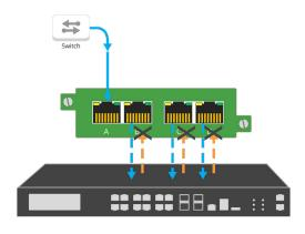
In this scenario you are able to ensure 1 SPAN port provides 1-3 copies of unidirectional traffic, without packet injection back onto the network.
