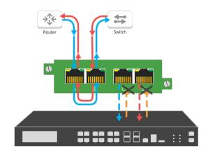
In this scenario you are able to TAP one link and provide unidirectional tap 'Breakout" copies of traffic, without packet injection back onto the network.
