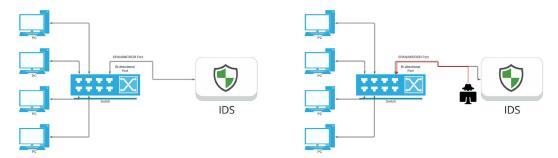
Utilizing "Data Diode" TAPs can remove all three of these vulnerabilities.
