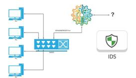
1. SPAN/Mirror ports involve management intervention and reconfiguration of the switches. This is not always a simple task (especially where VLAN's are also involved) and is prone to error.
