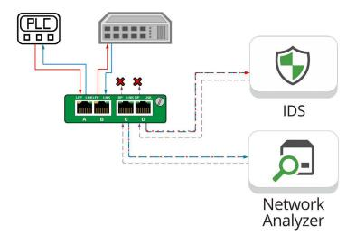
There are also some situations where the use of SPAN/Mirror ports is still needed for visibility. In these instances, it is "Best Practice" to connect the SPAN/Mirror port to a Data Diode TAP and use the TAP's SPAN/Regeneration mode to pass the mirrored SPAN data onto Monitoring/security devices. Using unidirectional Data Diode Taps in this way will ensure that there can be no data passed back into the Switch SPAN/Mirror port.
