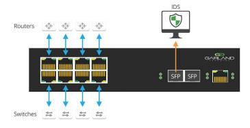
In this scenario you are able to TAP 4 links and provide unidirectional TAP copies of traffic aggregated to one or two ports, without packet injection back onto the network.
