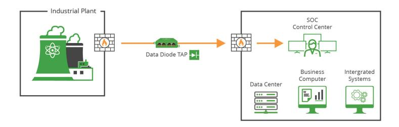
A network TAP creates an exact copy of both sides of the traffic flow, continuously 24/7/365 and does not drop packets, introduce delay, or alter the data. They are either passive or "failsafe," meaning traffic continues to flow between network devices if power is lost or a monitoring tool is removed, ensuring it isn't a single point of failure.
