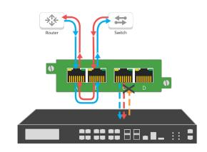
In this scenario you are able to TAP one link and provide unidirectional TAP copies of traffic aggregated to one or two ports, without packet injection back onto the network.
