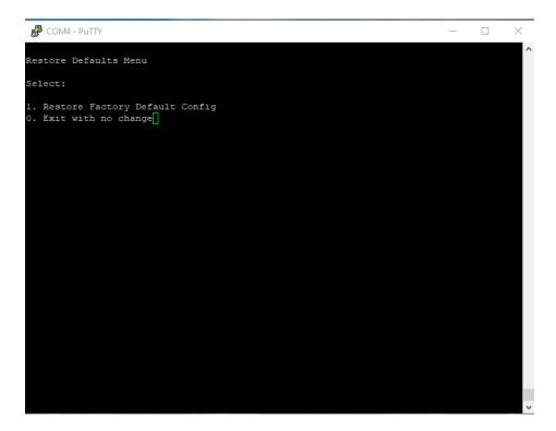
Note: A power cycle is required after pressing 1.
