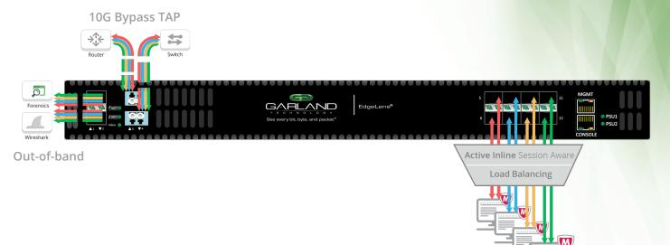
**Active In-Line Load Balancing** to multiple 1G NG-IPS
